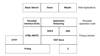
Fig. 2. Architectural components of the Prolog-based web-application
